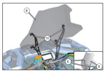
Align the holes on the front windshield (8) to the windshield brackets, then install the supplied M6x22 screws (6) and nuts (10). Tighten the fasteners sufficiently, using caution not to over-tighten.
