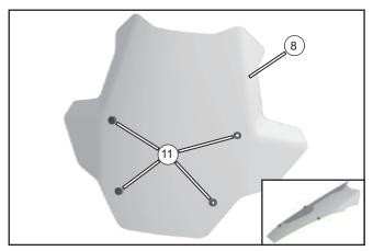
// Install the rubber bushings (11) into the corresponding holes on the front windshield (8).
