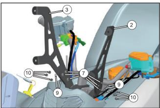
Align the corresponding holes of LH & RH windshield brackets A (2 & 3) to LH & RH windshield brackets B (4 & 5), then install M6×16 screws (7), washers (9), and nuts (10) in each hole and tighten them.
