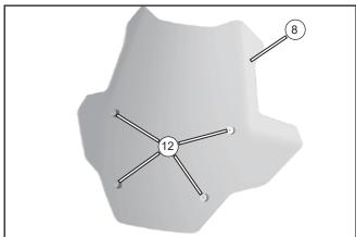
Install the rubber sleeve liners (12) into corresponding holes on the front windshield (8).
