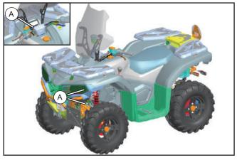
// Reinstall the handlebar guard (A).
