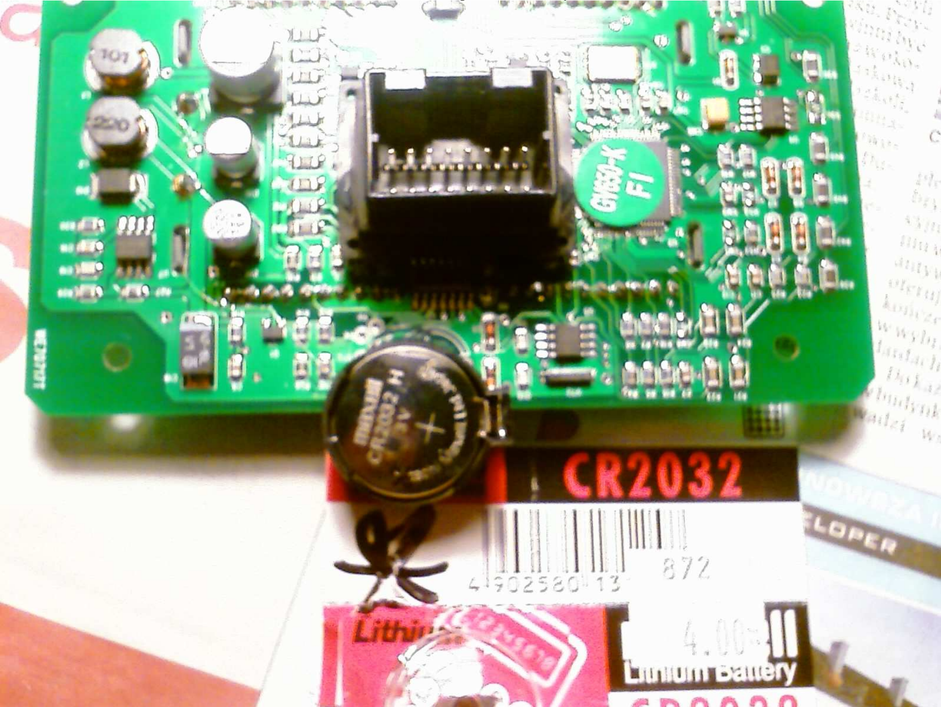
At the end we put a new battery.
